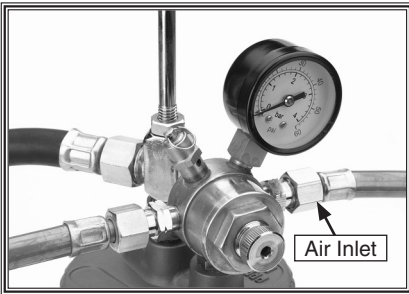
Figure 7. Compressed air inlet location.
